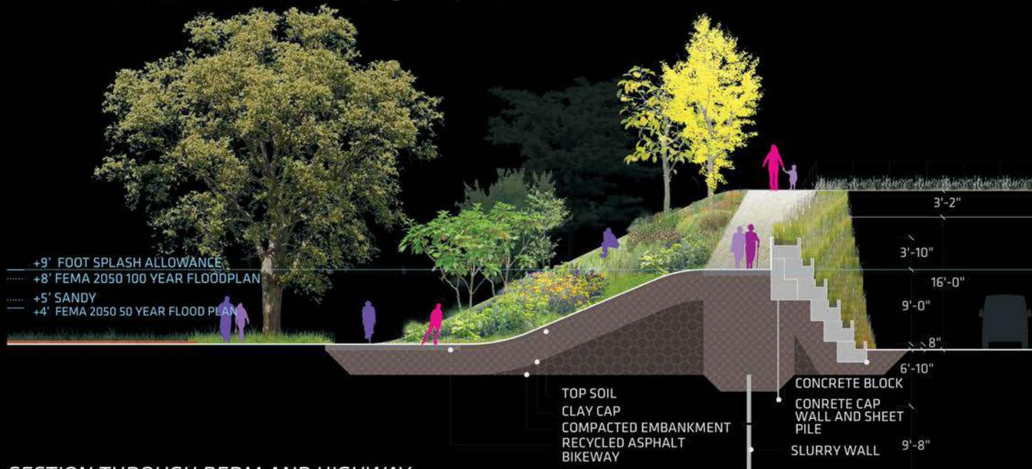
SECTION THROUGH BERM AND HIGHWAY
